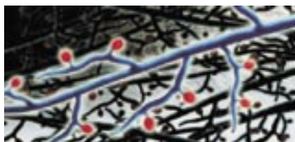
Representation of a section through the Smopex® fibre showing the high density of active functional groups in red
